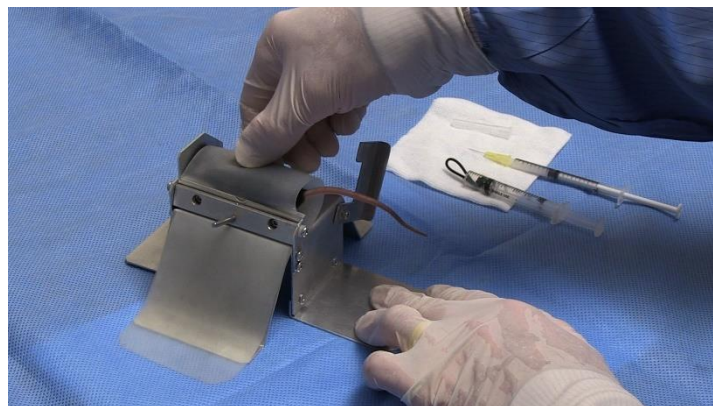
Figure 8: To release the mouse, unlock the tail gate, Unlock the membrane and allow mouse to exit the front or back of the device
